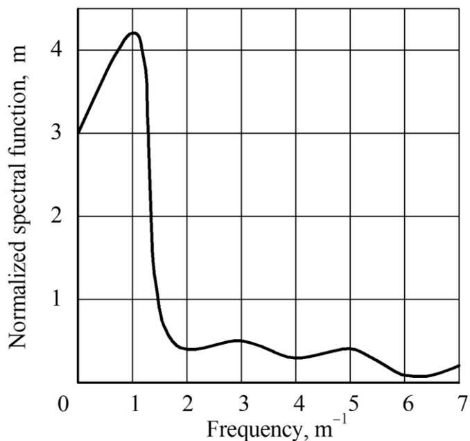
Fig. 7 - Spectral density of oscillations of the field surface longitudinal profile
