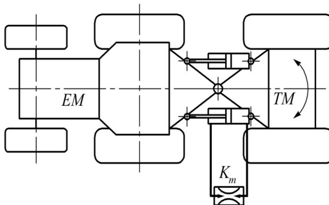
**Fig. 2 - An installation scheme of a throttle in the hydraulic cylinder, connecting the energy and the technological modules of the modular energy tool**
