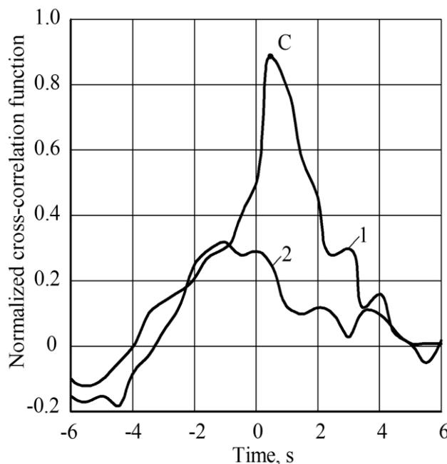
**Fig. 9 - The normalised mutual correlation functions of the relative bearing angle  $\varphi$  oscillations, caused by angle  $\alpha$  fluctuations at various throttling levels of the technological module's hydraulic cylinder**
