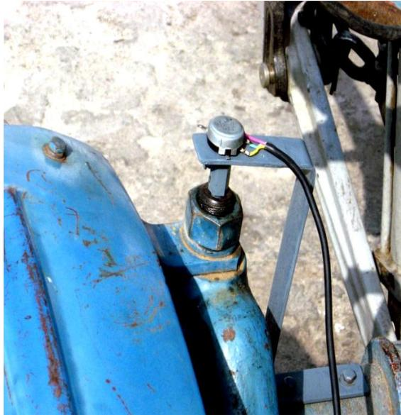
Fig. 4 - Resistor SP-3A (440 Ohm)
