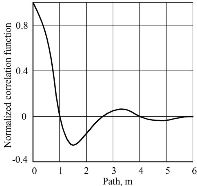
Fig. 6 - A normalised correlation function of oscillations of the field surface longitudinal profile
