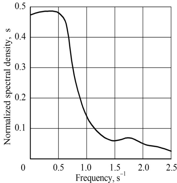
**Fig. 8 - Normalised spectral density of the turning angle oscillations of the modular energy tool's driven wheels**
