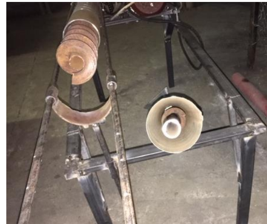
Fig. 3 - A stand for the study of telescopic screw conveyors in a disassembled state
