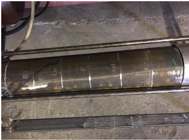
Fig. 2 - Scale of the stand screw to study the characteristics of telescopic screw conveyors
