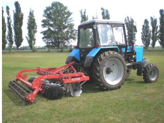
**Fig. 3 - General view of a disk header with spring shanks**
