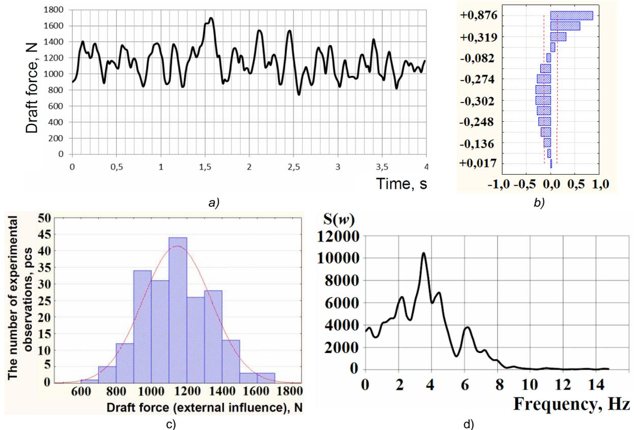
**Fig. 4 - Statistical characteristics of the interaction process of an operating element on a spring shank and the soil**
