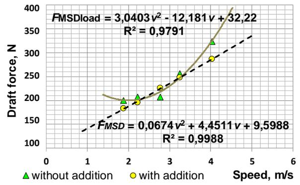
Fig. 6 - Mean-square draft force deviation-vs-unit travelling speed curve
