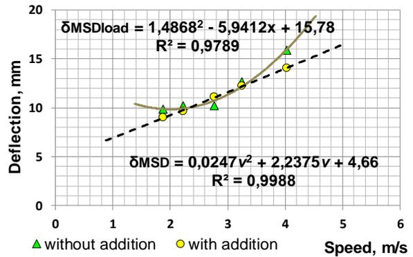
Fig. 8 - Mean-square value of shank deflections-vs-unit travelling speed characteristic curve  $\sigma = f(\delta)$
