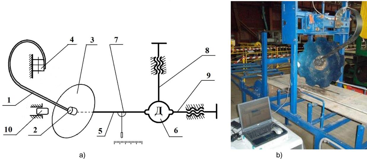
Fig. 1 - An experimental plant (technical equipment) for testing and evaluation of spring shank operation efficiency
