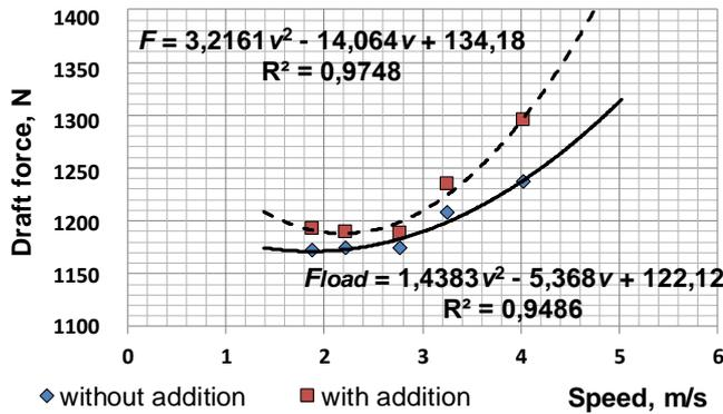
Fig. 5 - Draft force-vs-unit travelling speed characteristic curve (according to calibration curves)
