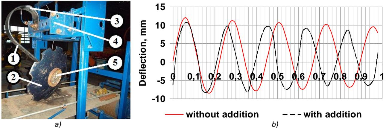
**Fig. 2 - Realization of laboratory investigations: a – exterior of a spring shank with ballast loading while determining the reduced mass; b – free spring shank oscillations**
