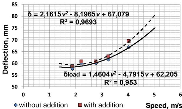
Fig. 7 - Average deflection value-vs-unit travelling speed curve (according to calibration curves)
