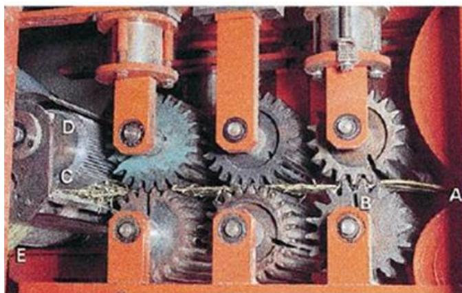
Fig. 2 - Working elements of the decorticator
