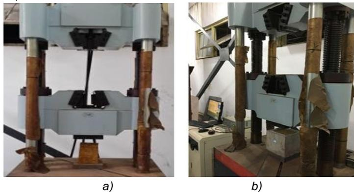
**Fig. 3 – Stress experiment of straw and composite bricks**
