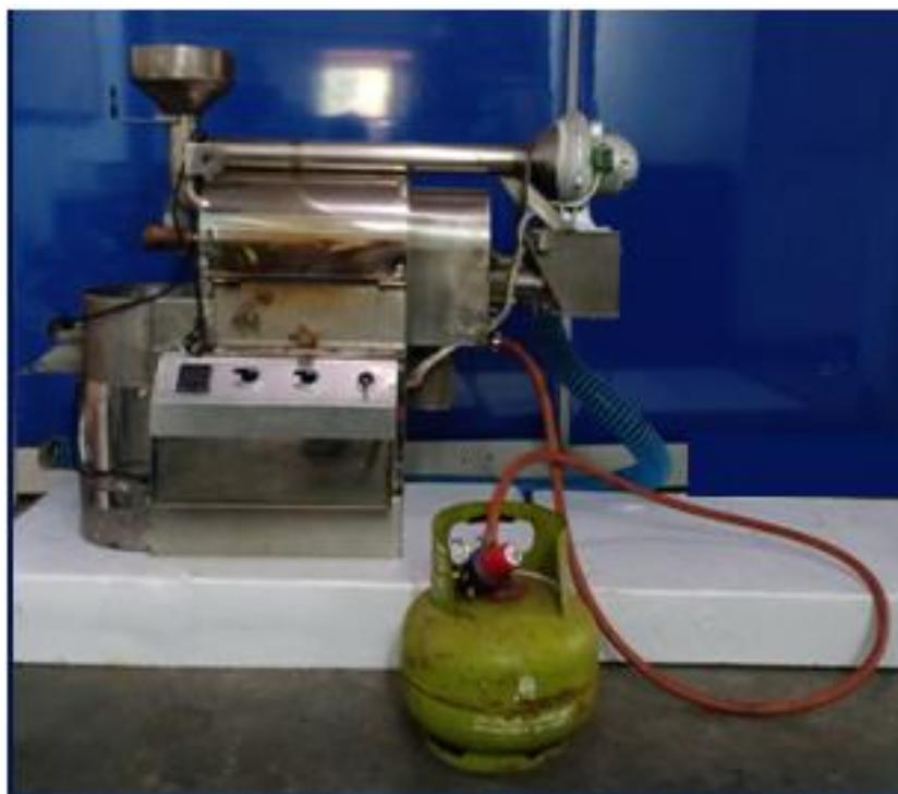
Fig. 4 - The prototype of a coffee roasting machine
