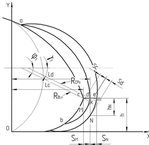
Fig. 5 – Diagram for determining the diameter of the onion harvester bed-shaping roller spiral drum
