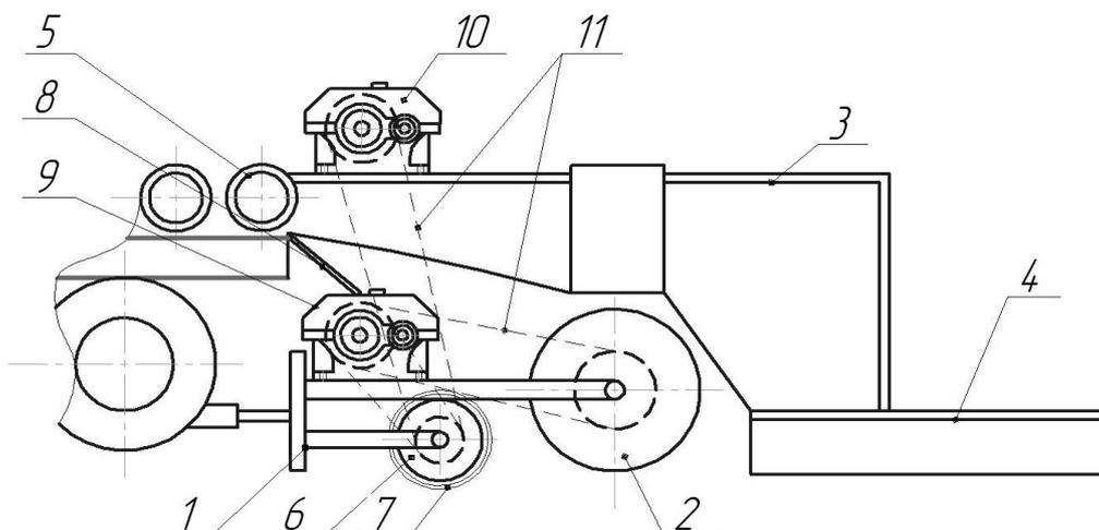
**Fig. 4 – Structure diagram of an onion harvester bed-shaping roller**
