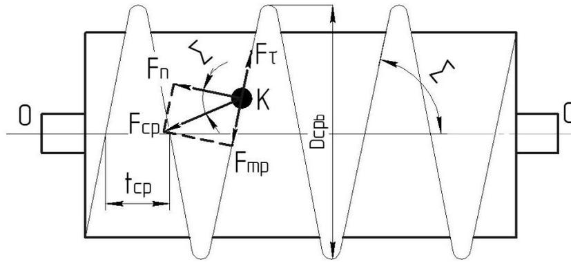
Fig. 7 – Diagram of the forces affecting a soil clump through the drum spiral
