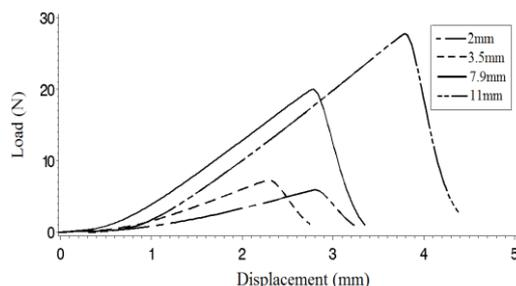
**Fig. 3 - Puncture force–displacement curves of peel with different probe diameters at 11 mm/s loading speed**
