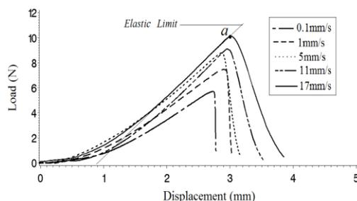
**Fig. 2 - Puncture force–displacement curves of peel with different loading speeds under 3.5 mm-diameter probe**
