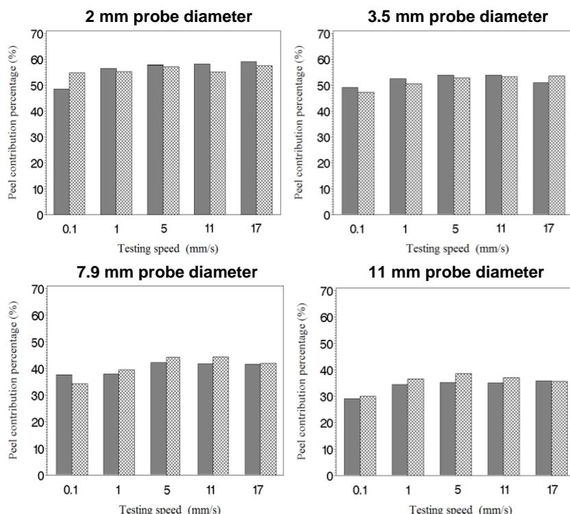
Fig. 6 - Peel contribution percentage to apple fruit firmness at different speeds
