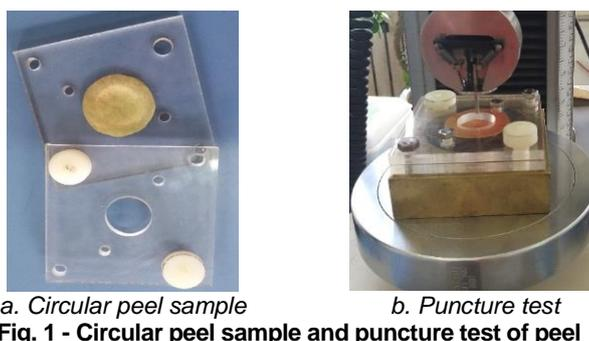
**Fig. 1 - Circular peel sample and puncture test of peel**
