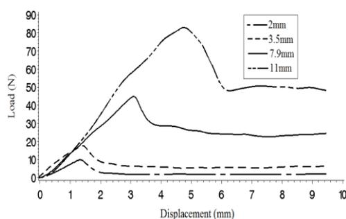
Fig. 5 - Puncture force–displacement curves of whole apples with different probes at 11 mm/s loading speed
