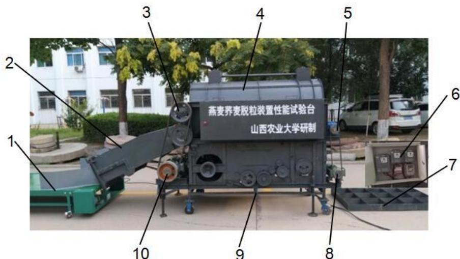
**Fig. 4 - Performance experiment unit of buckwheat threshing device**
