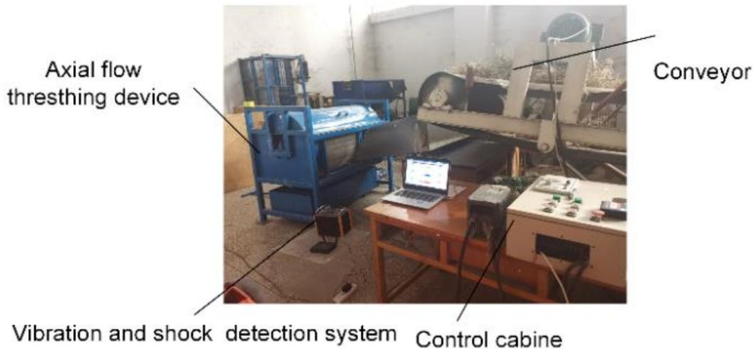
Fig. 6 – Test site of vibration and impact detection
