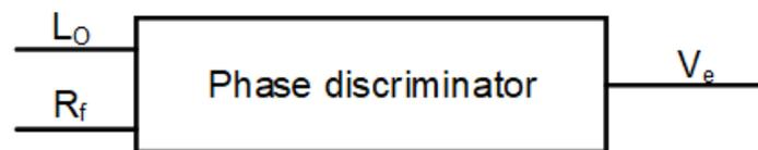
Fig. 5 - Principle block diagram of ideal phase discriminator
