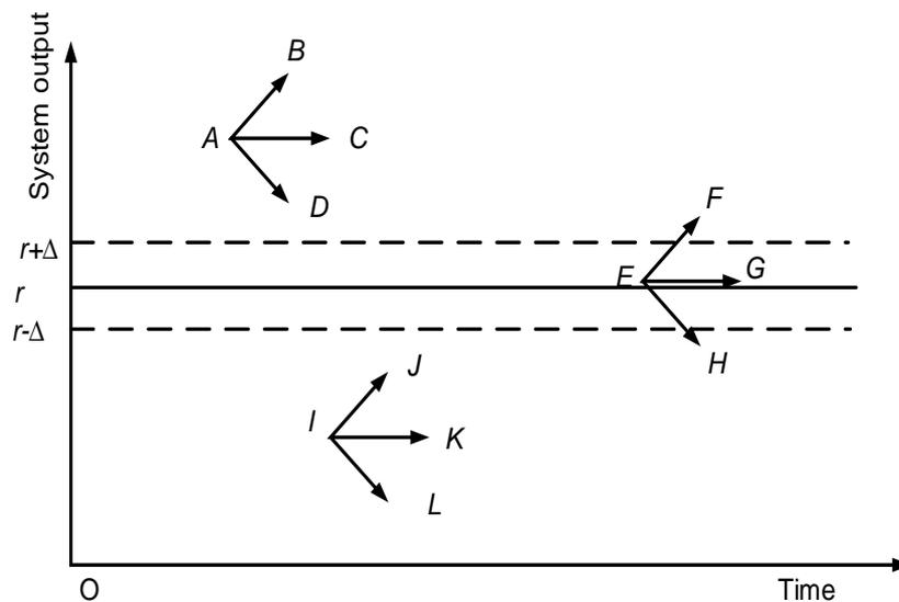
Fig. 1 - Nine-point controller system principle
