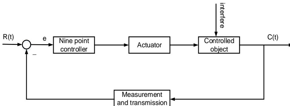
Fig. 2 - Schematic diagram of nine-point controller system
