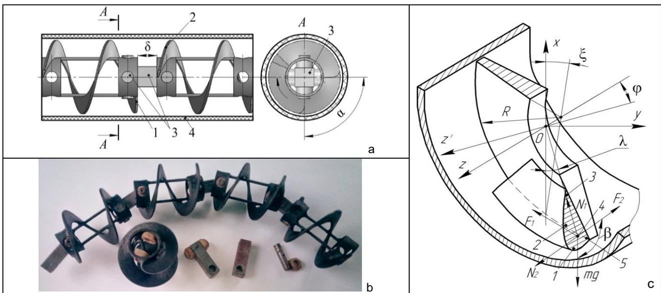
**Fig. 1 - Design and calculation scheme of the screw working body, the sections of which are hinged**
