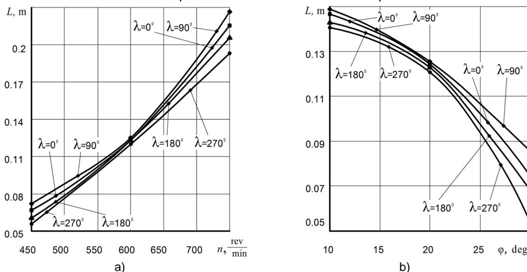
**Fig. 2 - Graphical dependences of the free flight range of the material particle  $L$  on the rotation speed of the working body  $n$  (a) and the angle of inclination of the screw section axis to the horizon (b) at different angular positions  $\lambda$  of the particle at the time of separation from the screw edge to contact with the lower surface of the casing**
