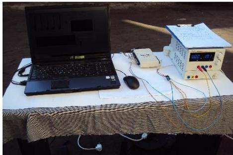
Fig. 14 - Data acquisition subsystem
