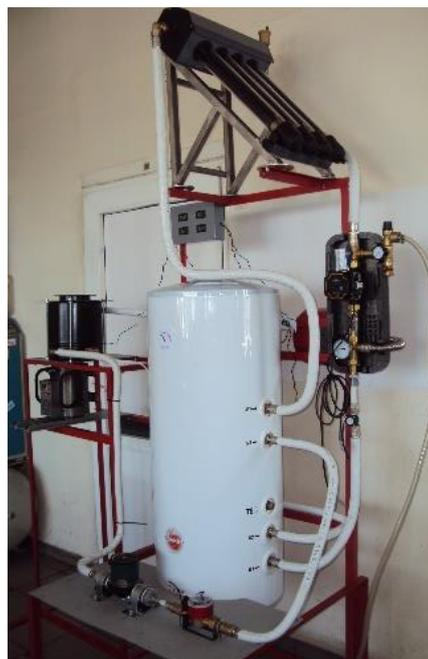
Fig. 2 - Physical development of the combined thermal system experimental model
