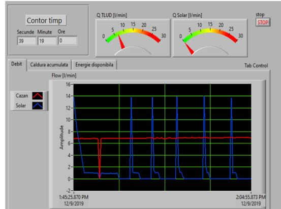
**Fig. 19 - Graph of variation of flow rates of circulation pumps**
