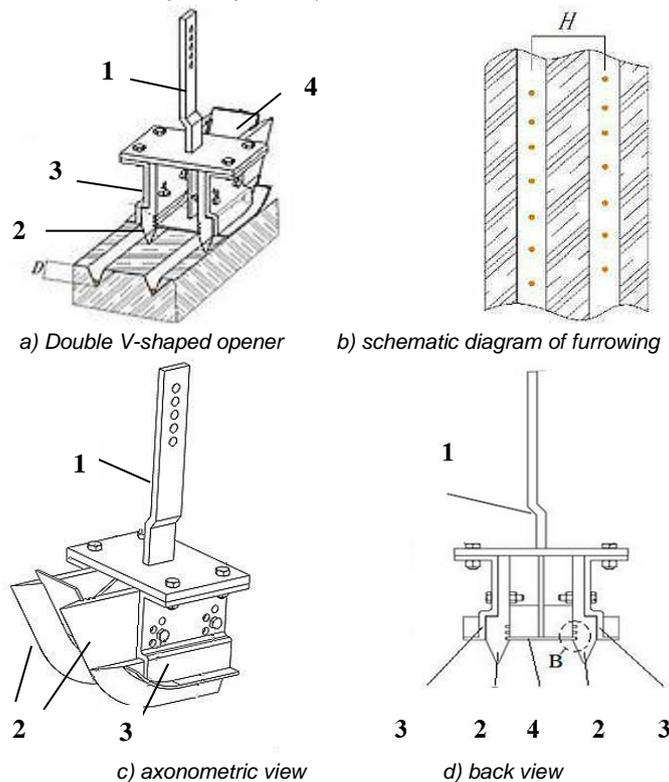
Fig. 2 - Double V-shaped opener
