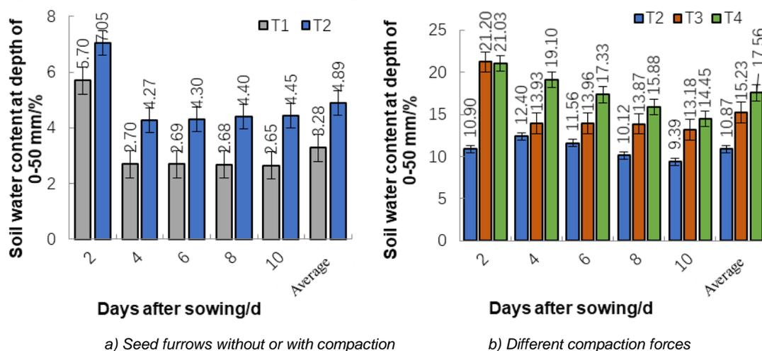
Fig. 5 - Effects of different operating method on soil moisture content at the depth of 0-50 mm
