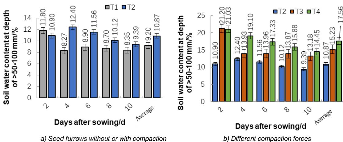
Fig. 6 - Effects of different operating method on soil moisture content at the depth of >50-100 mm
