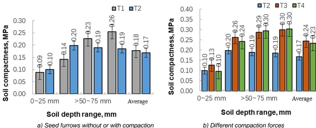
Fig. 8 - Effects of different treatments on soil compactness
