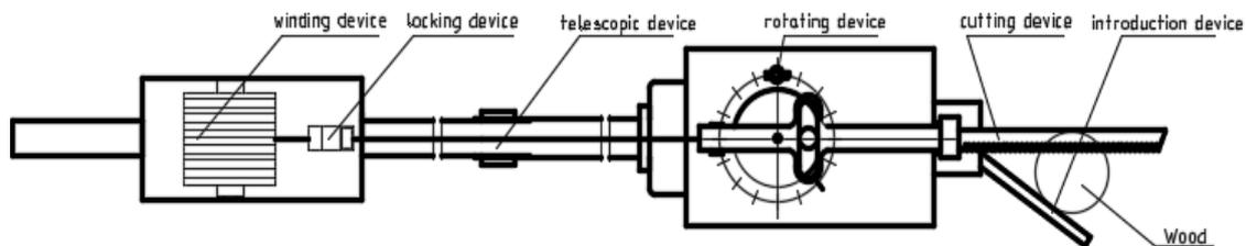
Fig. 1 - Schematic diagram of omni-directional pruning saw
