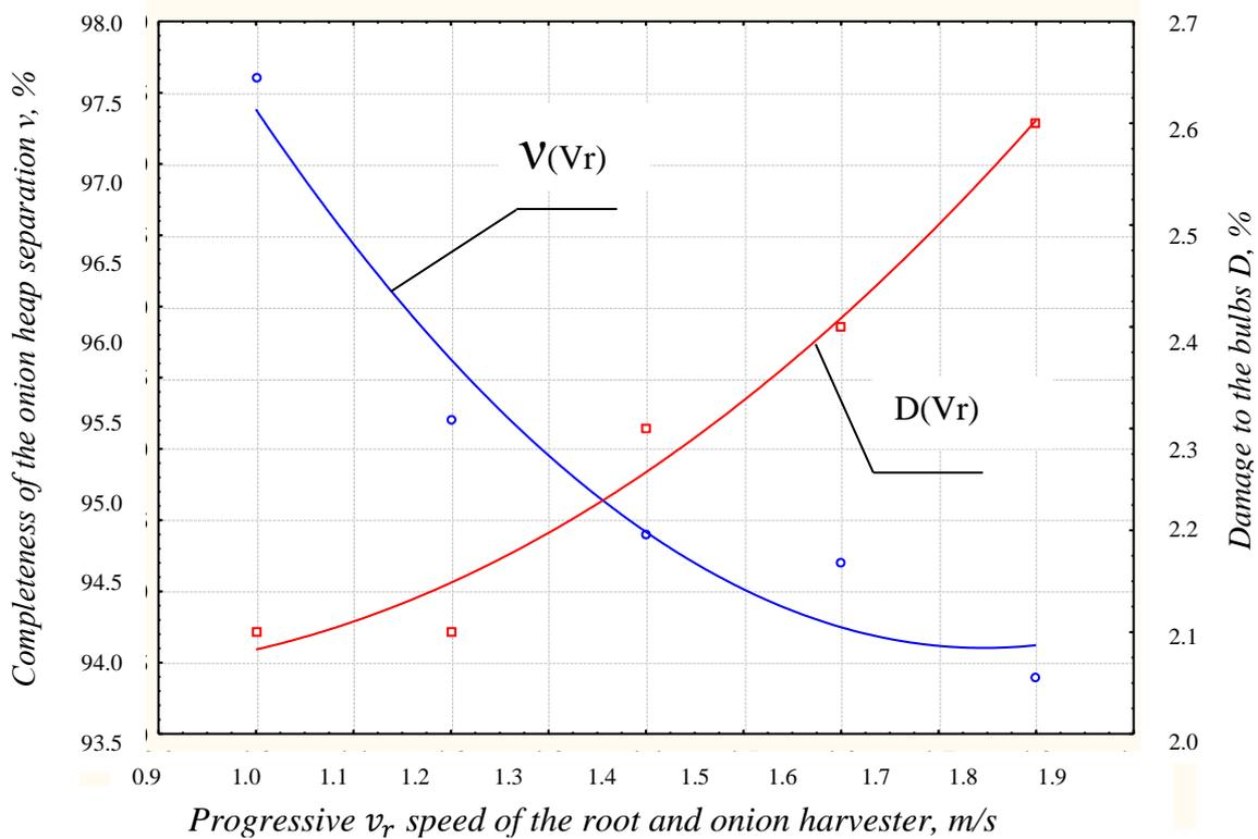
**Fig. 5 – Dependence of the completeness of separation  $v$  and damage to bulbs  $D$  of separating rod elevator with adjustable blade inclination angle vs. the progressive  $v_r$  speed of the root and onion harvester**
