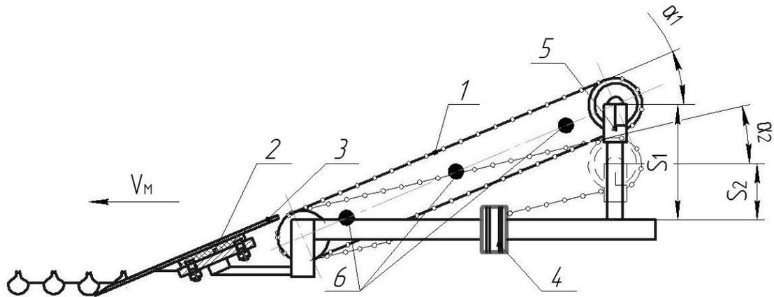
**Fig. 1 – Diagram of changes in the inclination angle of the rod elevator:**
