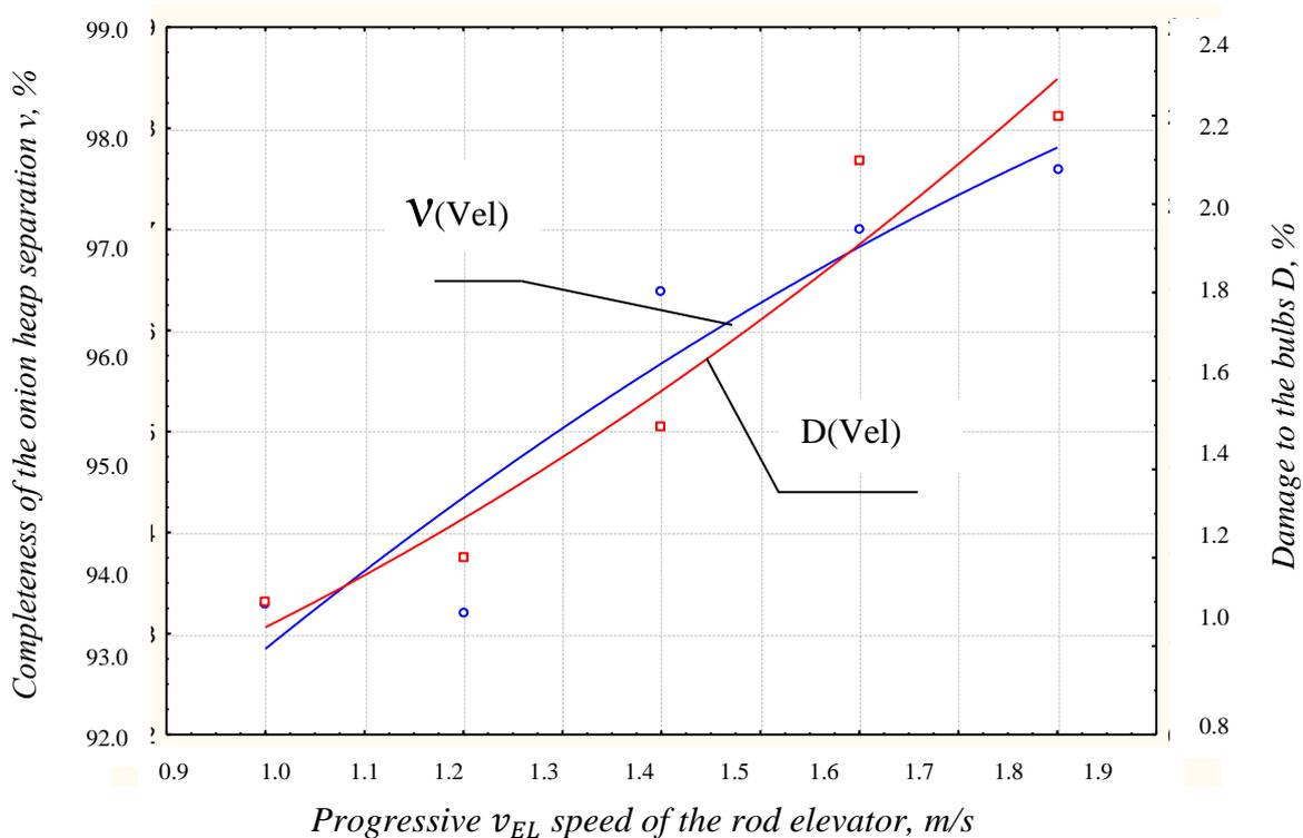
Fig. 6 – Dependence of the completeness of separation  $v$  and damage to bulbs  $D$  of separating rod elevator with adjustable blade inclination angle vs. the progressive speed  $v_{EL}$  of the rod elevator blade
