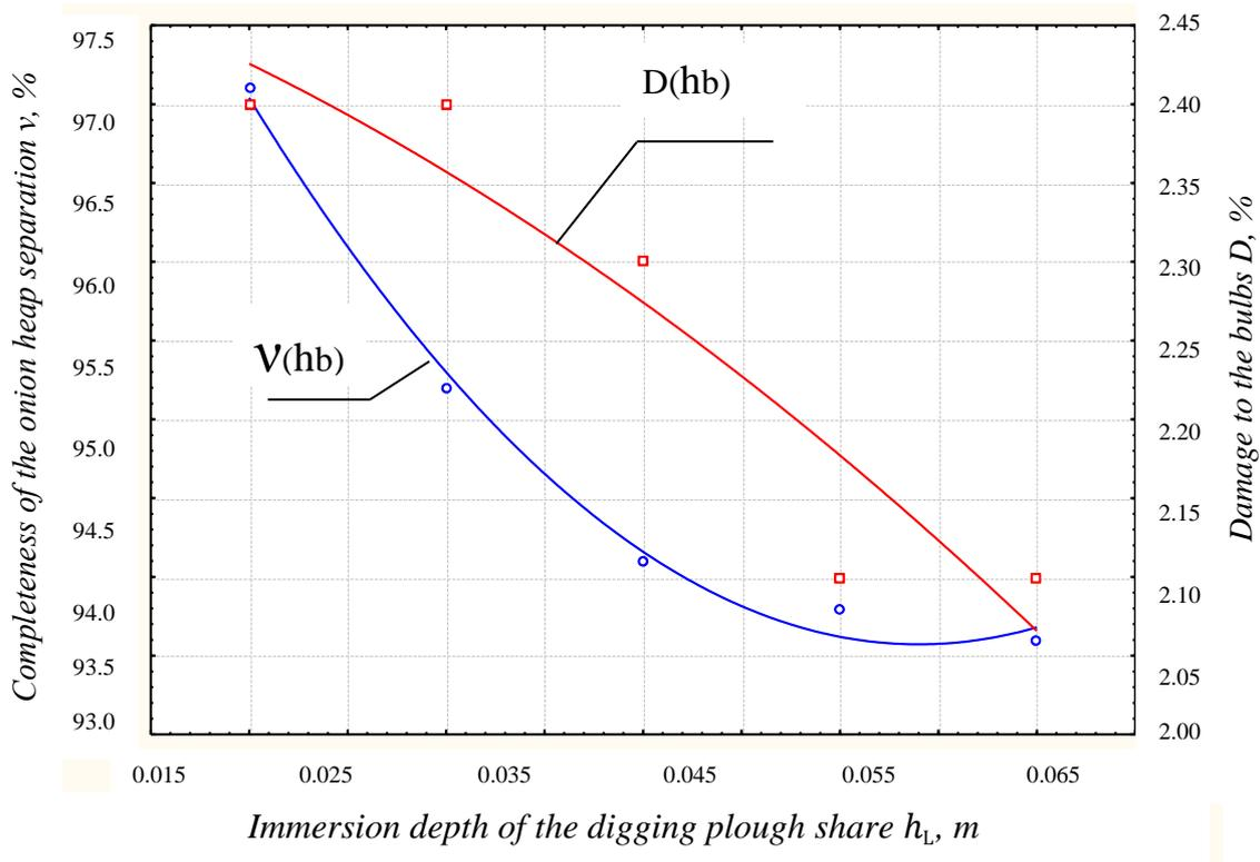
**Fig. 4 – Dependence of separation completeness  $v$  and damage to bulbs  $D$  of a separating rod elevator with an adjustable blade inclination angle vs. depth  $h_L$  of the digging plough share immersion into the soil**
