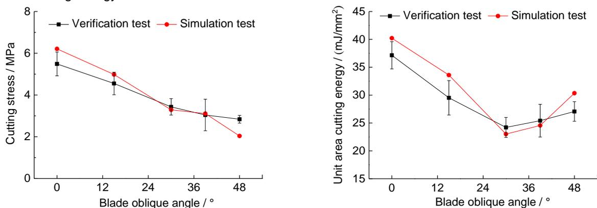
Fig. 11 - Variation of cutting mechanical properties with blade oblique angle
