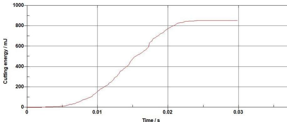
Fig. 9 - Curve of cutting energy with time of inner tissue of stalk in simulation test
