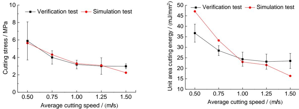
Fig. 10 - Variation of cutting mechanical properties with cutting speed
