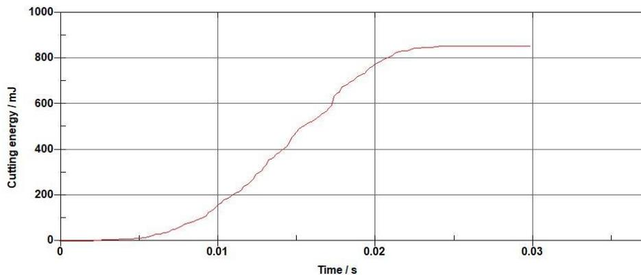
Fig. 8 - Curve of cutting energy with time of epidermal tissue of stalk in simulation test
