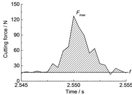
Fig. 4 - Curve of cutting force with time of millet stalk in verification test
