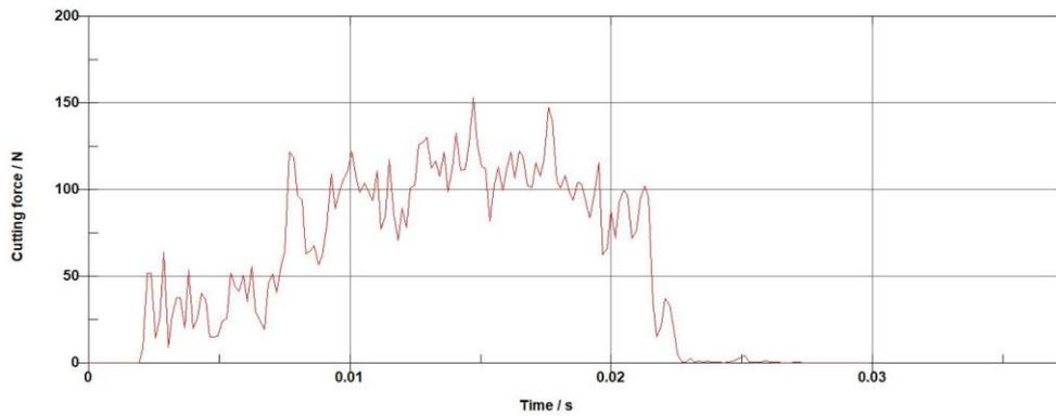
Fig. 7 - Curve of cutting force with time of millet stalk in simulation test
