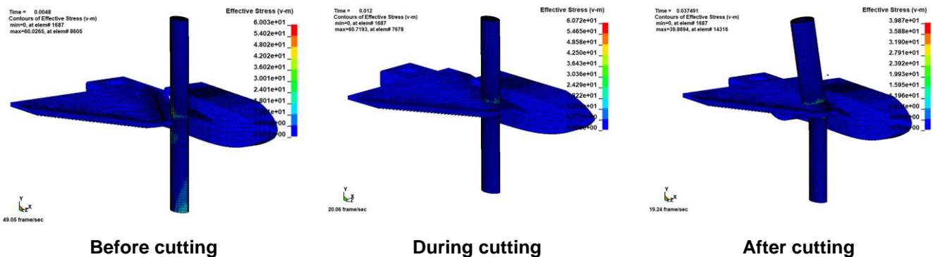
Fig. 6 - Stress and strain cloud diagram of the millet stalk during cutting
