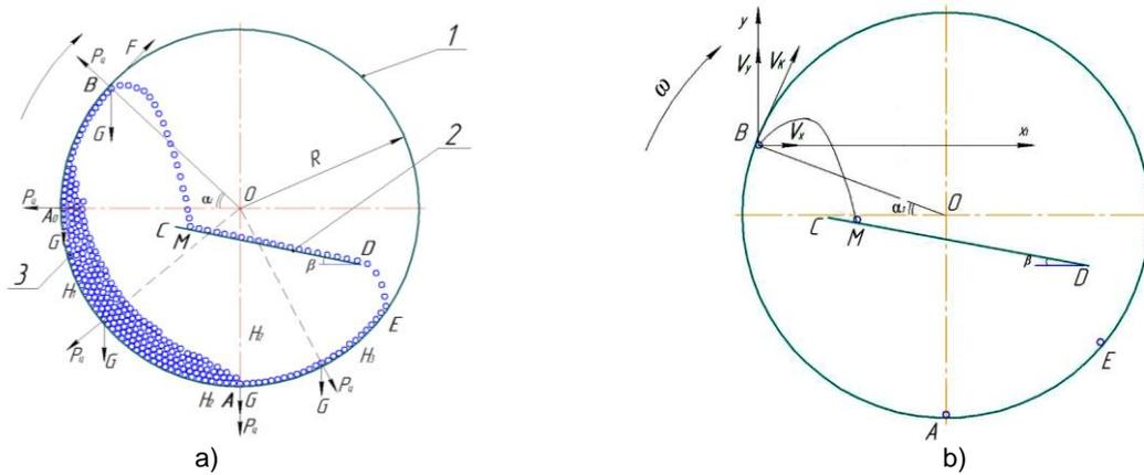
Fig. 3 - The scheme of the seed coating machine and the various positions of the capsules:
