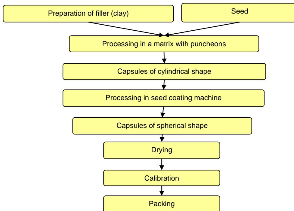
Fig. 1 - Technological scheme of obtaining encapsulated seeds
