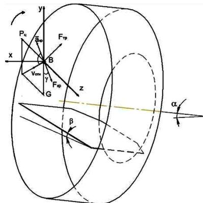
Fig. 4 - The calculated scheme of the forces of seed coating machine at an angle to the horizon and the flight path of the capsule
