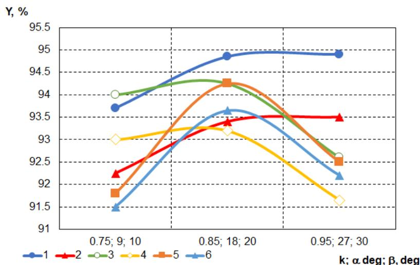
**Fig. 8 - Comparison of experimental data with theoretical ones (dependence of the dynamic indicator of the seed coating machine  $k$ , the angle of drum installation, the angle of the slope board installation from  $Y$ , %:**
