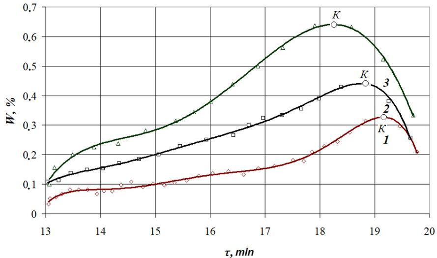
**Fig. 2 - Effect of the coolant temperature on the barley seeds drying rate**
