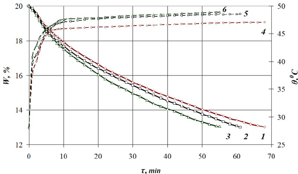
**Fig. 7 - Influence of the heating medium movement rate and the material heating temperature on the barley seeds drying duration:**
