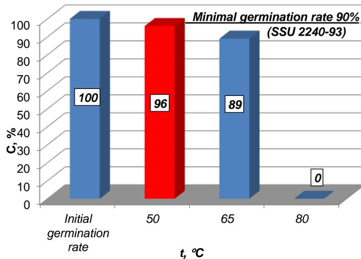
**Fig. 3 - Effect of the coolant temperature on the germination rate of barley seeds on the 7th day of germination:**  $V = 1.5 \text{ m/s}$ ,  $W_n = 20\%$ ,  $d = 10 \text{ g/kg d.a.}$
