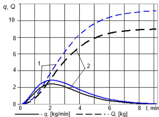
Fig. 7 – Graphs of simulation of  $q$  milk ejection intensity and  $Q$  milk quantity by simulator of milk ejection intensity during the cow milking period
