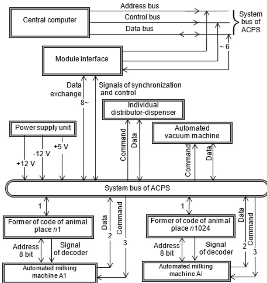
Fig. 1 – Structural scheme of adaptive cyber-physical system of milk production
