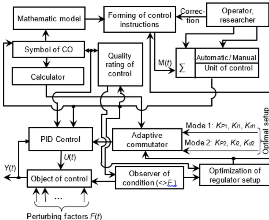
Fig. 5 – Functional scheme of the adaptive control module with search (expert) self-tuning system
