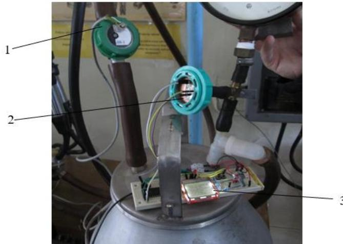
**Fig. 8 – General view of the measurement system of vacuum gage pressure fluctuation**
