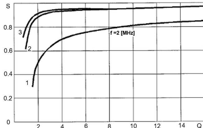
**Fig. 12 – Dependence of the differential sensitivity of the converter on its Q-factor**
