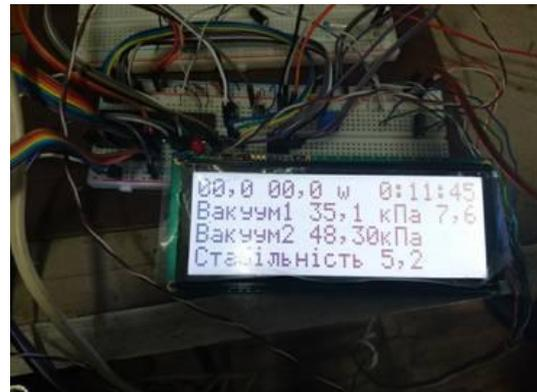
**Fig. 10 – General view of the microprocessor unit of the adaptive milking machine**
