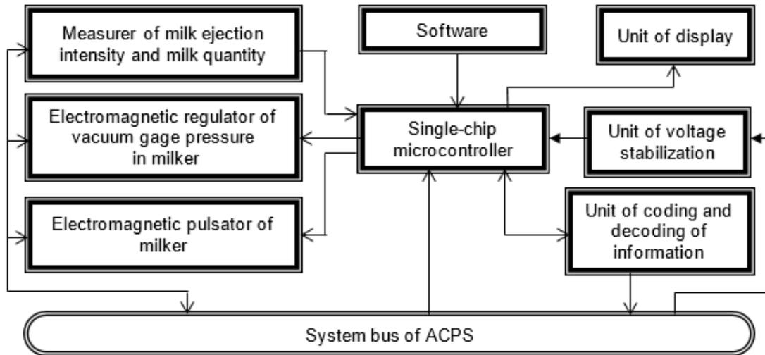
Fig. 3 – The structural chart of an adaptive milking machine as to the ACPS
