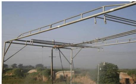
Fig. 3 - Pictures of direct injection-type rainfall simulator
