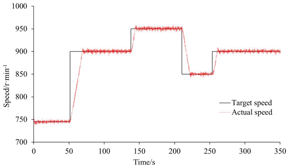
**Fig. 5 - Fan speed tracking**
