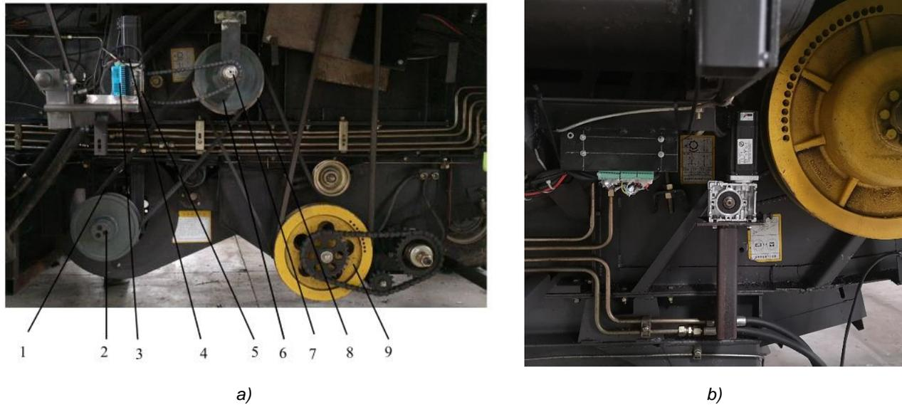
**Fig. 1 - Stepless speed regulating mechanism**
