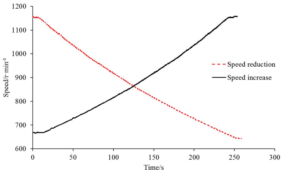
**Fig. 4 - Threshing cylinder speed regulation curve**
