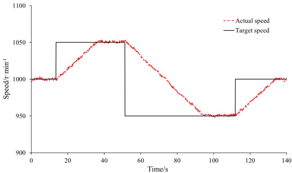
Fig. 6 - Threshing cylinder speed tracking
