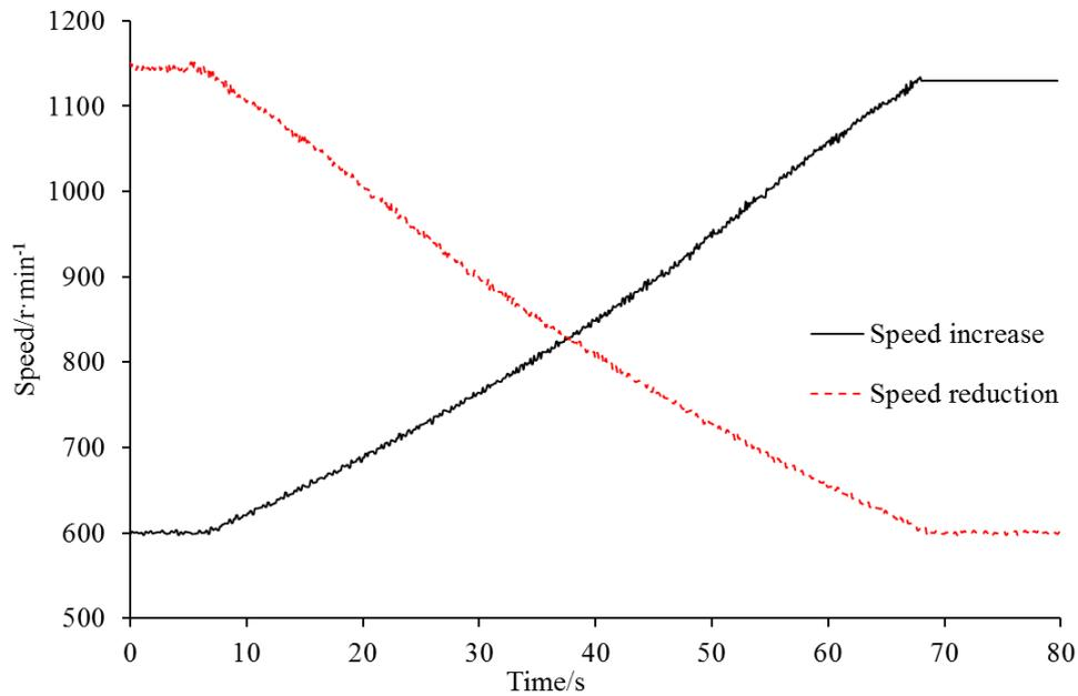
**Fig. 3 - Fan speed regulation curve**
