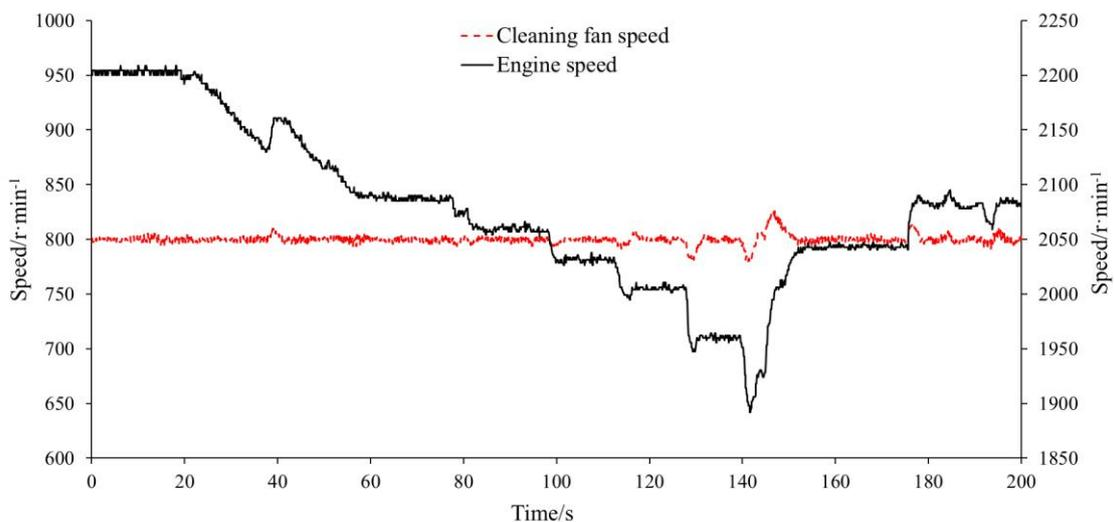
Fig. 7 - Fan speed during sudden load changes
