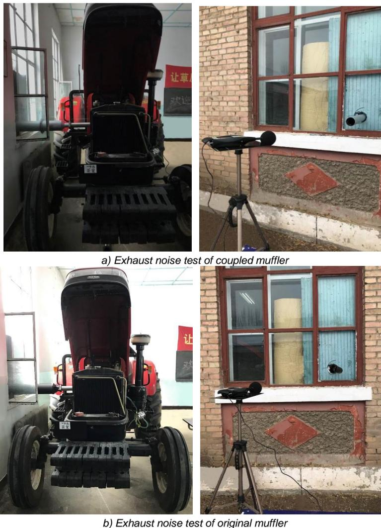
**Fig. 3 - Photos of insertion loss test for mufflers**
