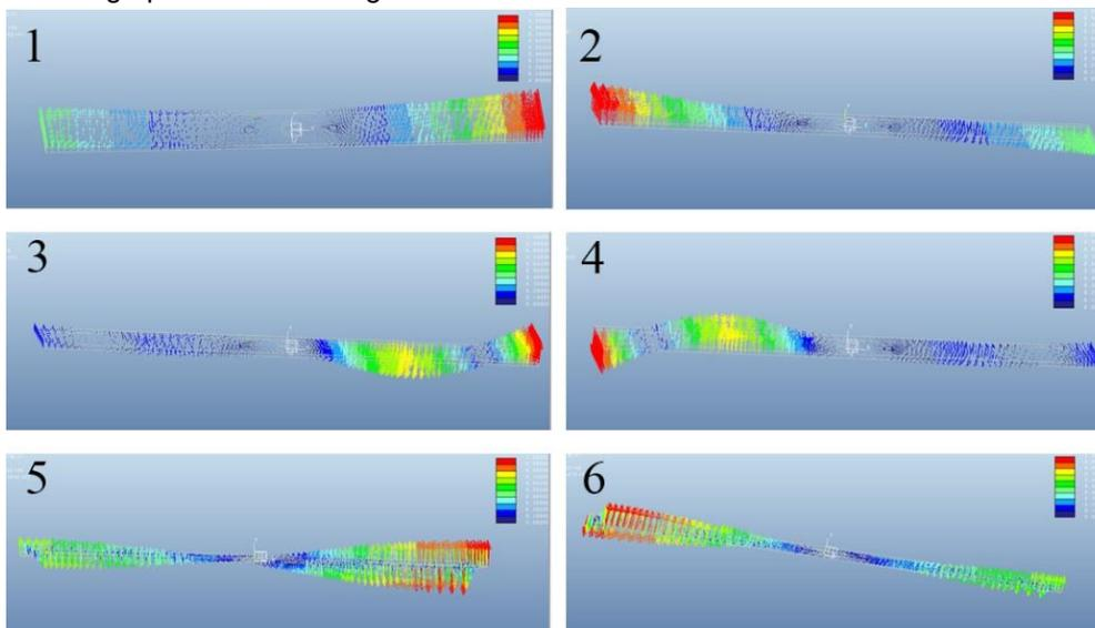
Fig. 7 – Vibration patterns of cutting blades
