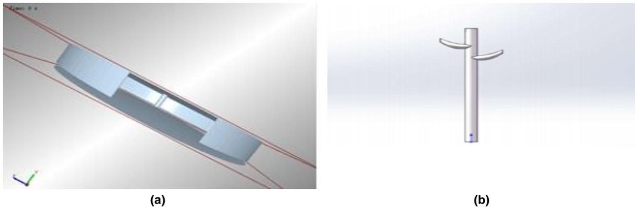
Fig. 3 – Geometric model: (a) Grass box and cutting blades; (b) Grass
