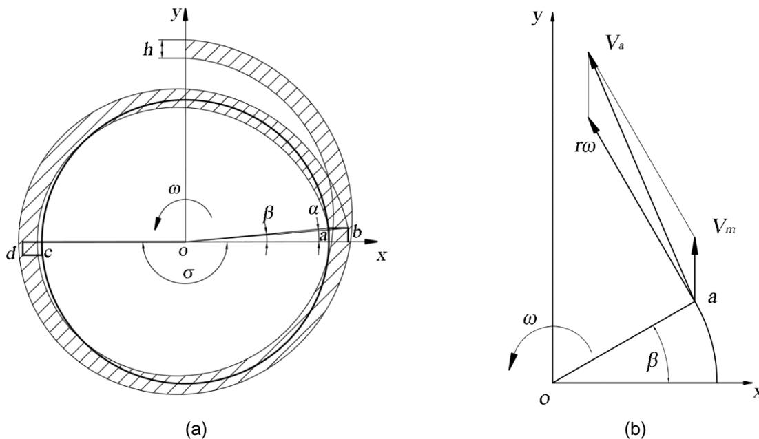
Fig. 2 – Trajectories of end points of cutting-edge and cutting velocity: (a) trajectory; (b) cutting velocity
