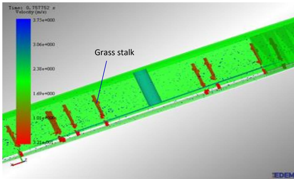
Fig. 4 – Contour of velocity of typical particles of grass
