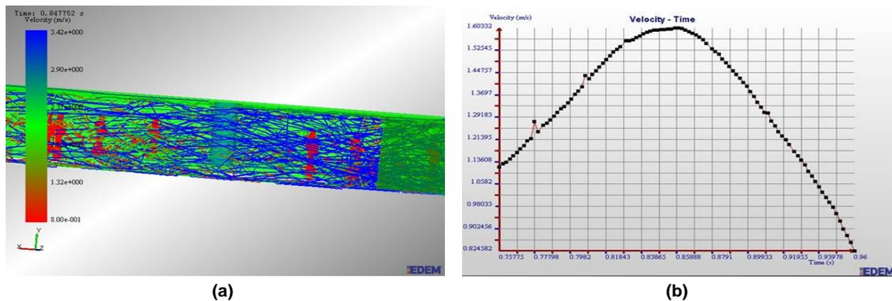
Fig. 5 – Typical particle move: (a) Grass trajectory; (b) Velocity vs. time
