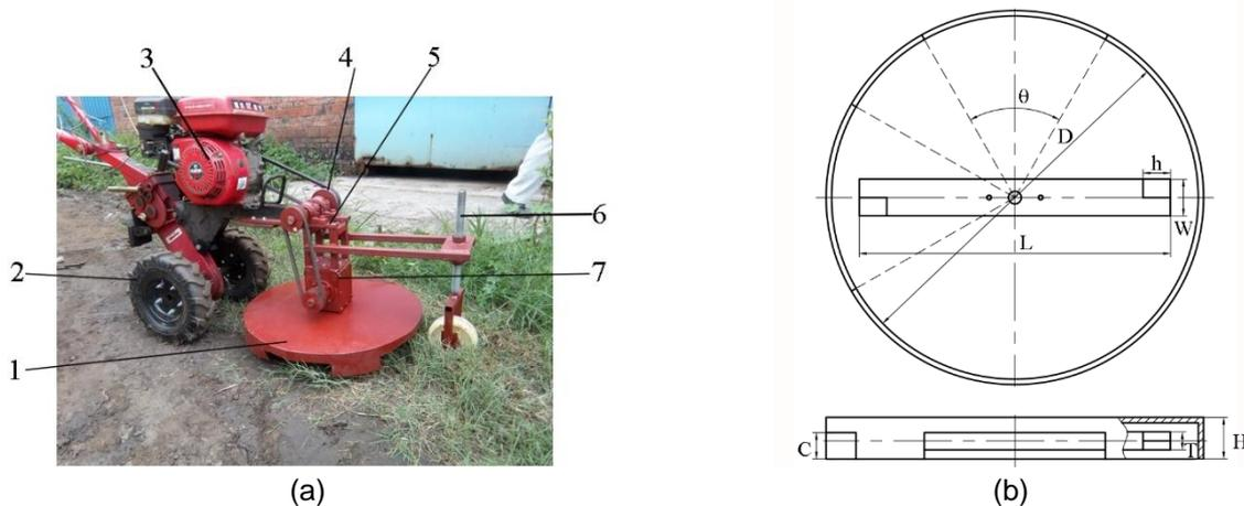
**Fig. 1 - Lawn mower: (a) outlook; (b) dimensions of grass box and cutting blades**
