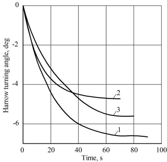
Fig. 8 - Dynamics of the angle of rotation of the harrow section with different offsets of its leashes' attachment point: 1 –  $d = 0$ ; 2 –  $d = 0.10$  m; 3 –  $d = 0.20$  m
