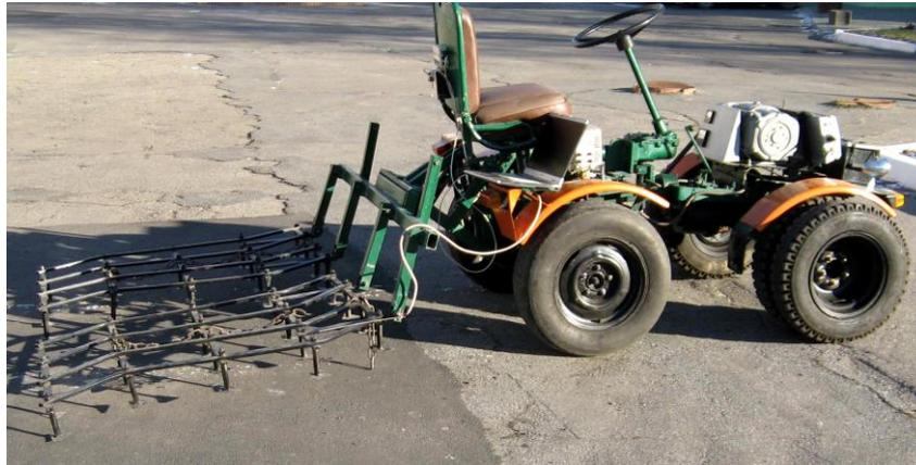
Fig. 3 - The harrow aggregate, composed on the basis of an electrical mini tractor
