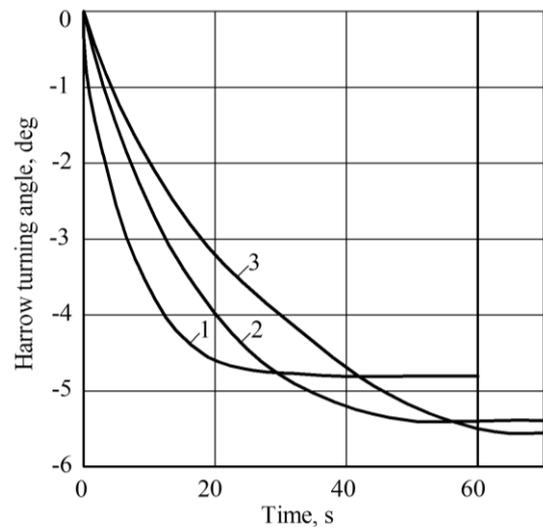
Fig. 7 - Dynamics of changes in the angle of rotation of the harrow section at different distances between the rows of its teeth: 1 –  $b = 0.15$  m; 2 –  $b = 0.30$  m; 3 –  $b = 0.45$  m
