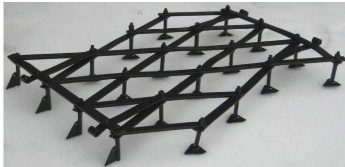
Fig. 1 - The harrow section of a new design
