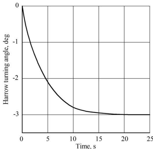
Fig. 10 - Dynamics of the angle of rotation of the harrow section with rational values of its design parameters
