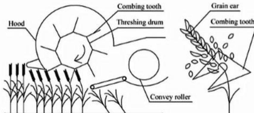
Fig. 3 - Pre-cut combing threshing harvester (Fu et al., 2018)
