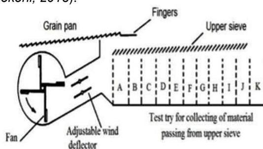
Fig. 2 - A schematic diagram of a cleaning mechanism (Mirzazadeh et al., 2015)
