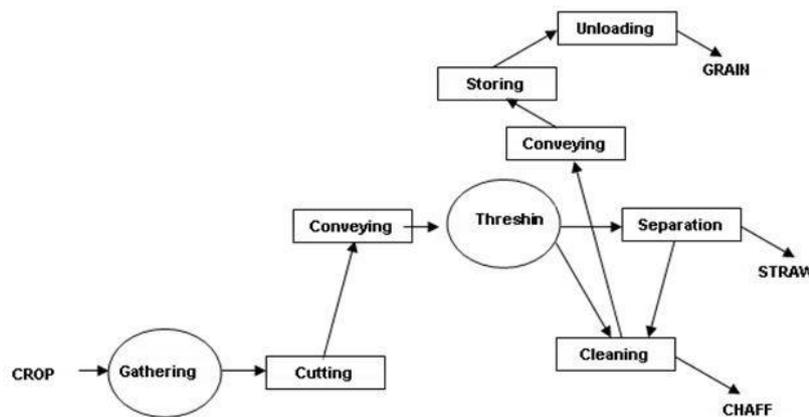
Fig. 1 - A simplified flow chart of the internal tasks of a combine harvester (Keskin and Şekerli, 2018)
