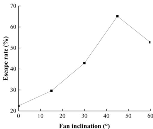
Fig. 6 - Escape rate on the circular sieve as a function of fan inclination
