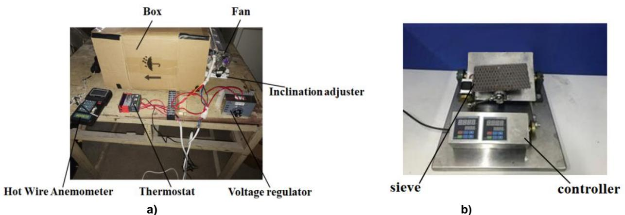
Fig. 3 - Test equipment
