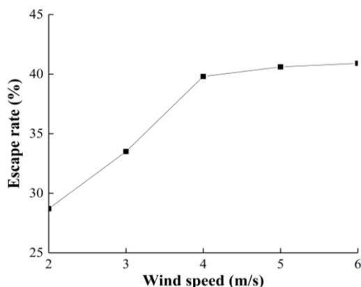
Fig. 5 - Escape rate on the circular sieve as a function of wind speed
