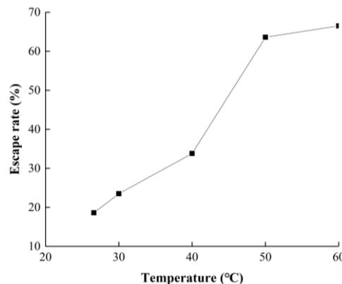
Fig. 4 - Escape rate on the circular sieve as a function of temperature
