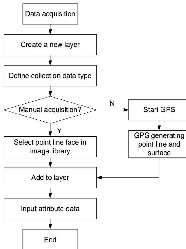
**Fig. 5 - Flow chart of data acquisition module**
