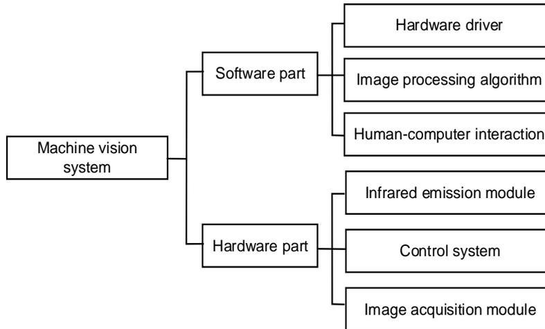
**Fig. 1 - Frame diagram of machine vision system**
