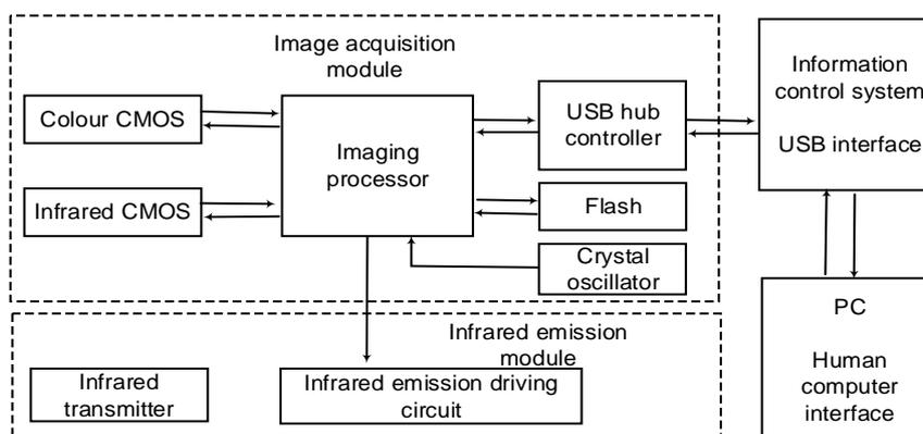
**Fig. 2 - Hardware architecture of machine vision system**
