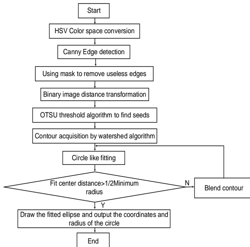
**Fig. 5 - Watershed algorithm flow based on Canny edge detection**
