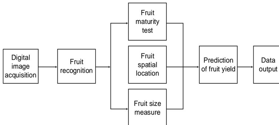
**Fig. 3 - Software architecture of machine vision system**
