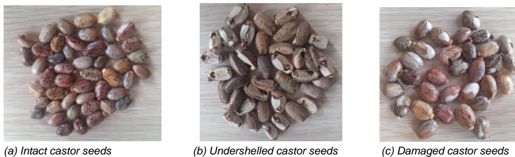
Fig. 10 - Shelling effect of the testbed
