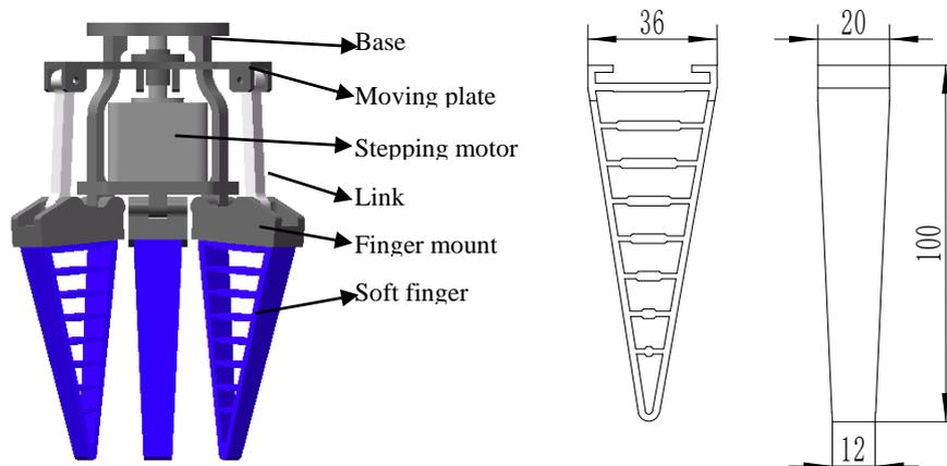
Fig. 1 - Schematic drawing of end-effector structure (a) and the soft finger (b)
