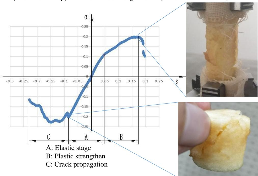
Fig. 6 - The stress-strain curve of the apple cortex during the tensile test and compression test
