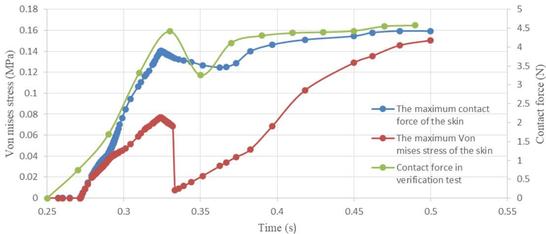
Fig. 9 – Simulation results of the maximum Von Mises stress and maximum contact force of the apple skin
