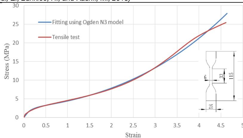
Fig. 5 - Strain-stress curve of the tensile tests and fitting using the Ogden N3 model of the TPU specimen
