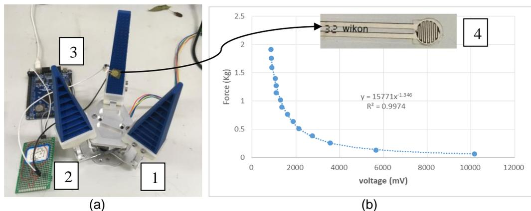
**Fig. 4 - Schematic diagram of the test device (a) and voltage and pressure diagram after calibration (b)**
