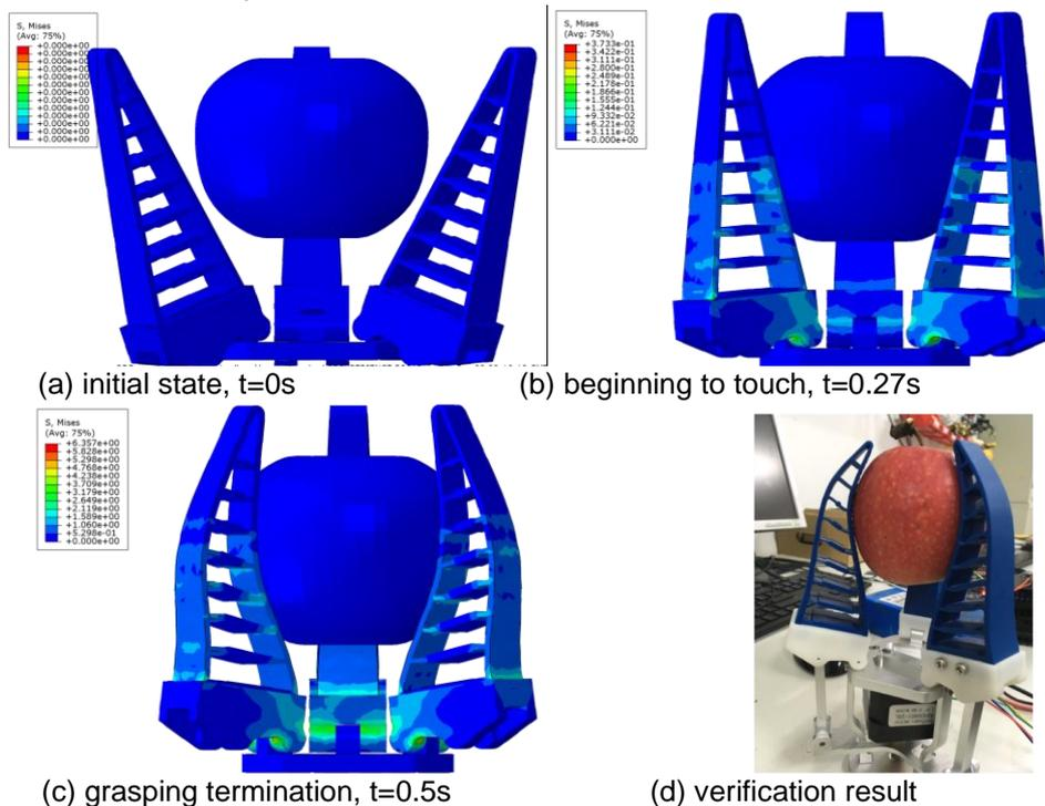
Fig. 8 - Stress cloud diagram of the grasping process of the end-effector in the simulation and verification test
