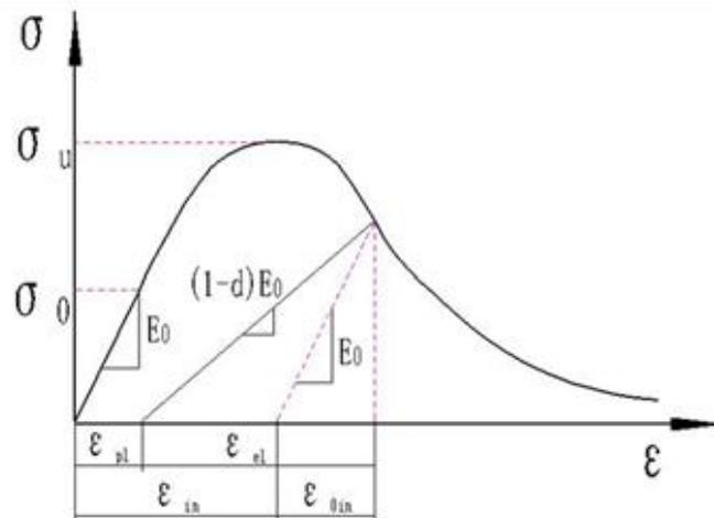
Fig. 3 - Schematic diagram of damaged-plasticity model
