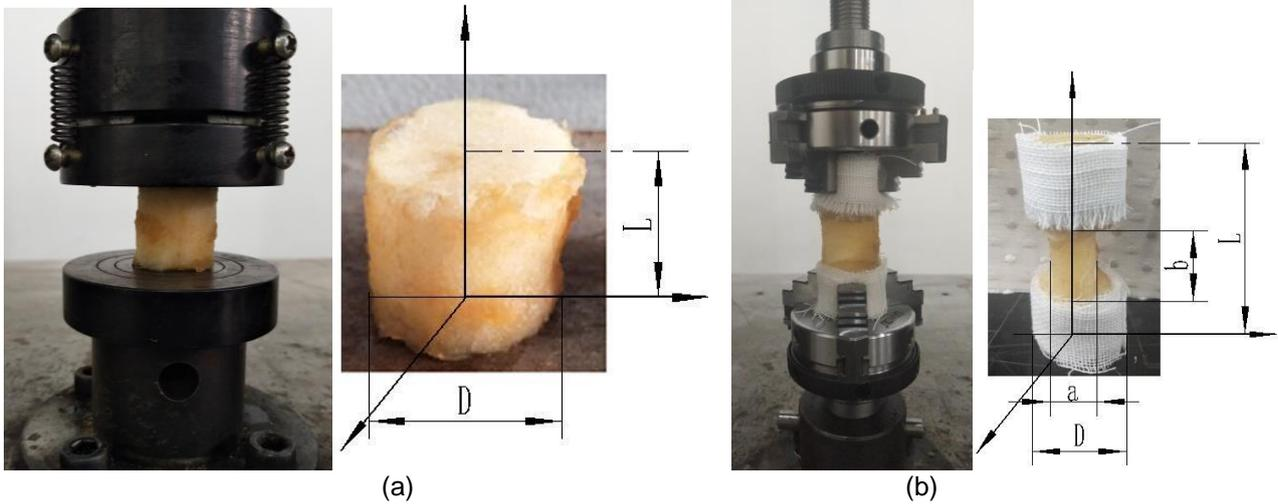
Fig. 2 - Cortex samples for compression test (a) and tensile test (b)
