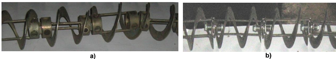
Fig.9 - Sectional screw operating members with a) hinged joints; b) safety joints
