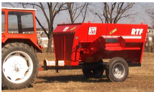
Fig.1 – Technological trailer for chopping, transporting and distributing the forage, RTF
