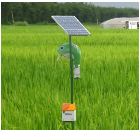
Fig.1 - Acquisition system of rice planthopper images
