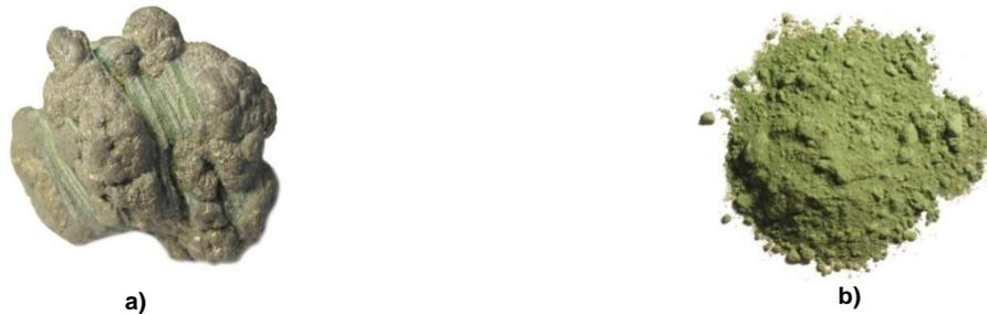
**Fig. 3 - glauconite before and after grinding**
