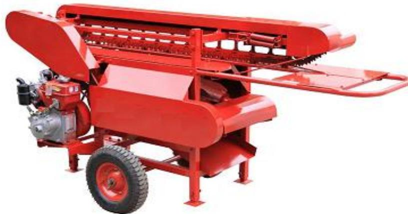
Fig.1 - Structure diagram of the peanut picking device
