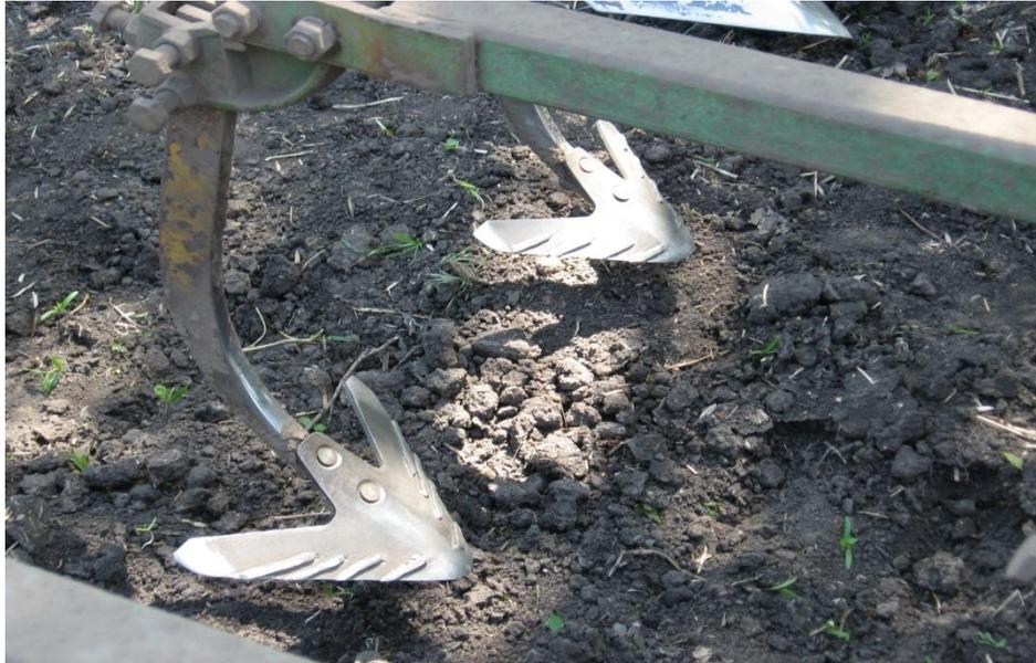
Fig. 4 - Experimental samples of sweeps
