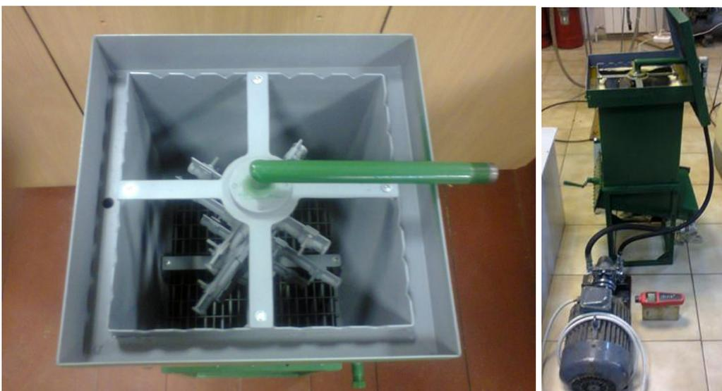
**Fig. 2 - General view of the experimental model of the hydro-mechanical mixer**
