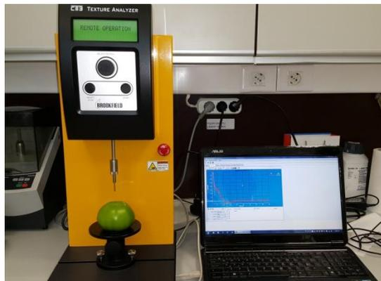
Fig. 1 - Texture analysis device and puncture test
