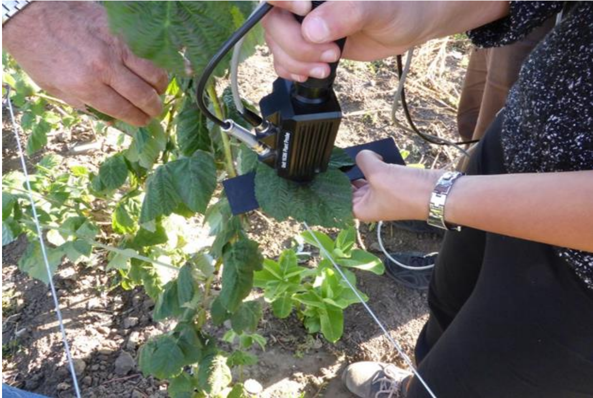
Fig. 6 – Contact reflectance measurement with PlantProbe
