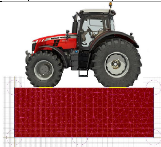
Fig.3 - Meshed model of soil used to analyze the distribution of stresses and strains in the longitudinal-vertical plane
