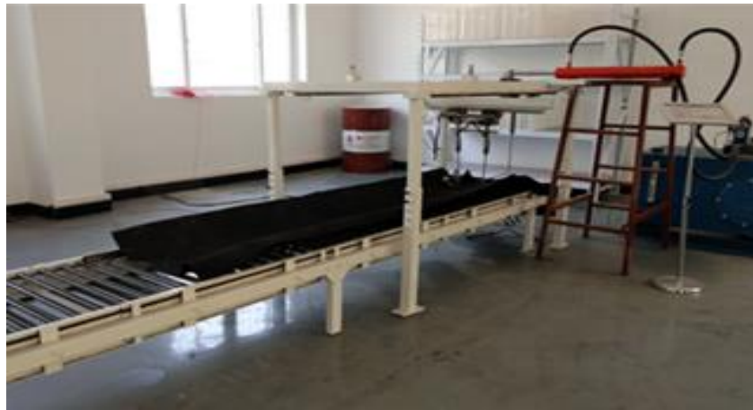
Fig. 10 - The automatic alignment test bench of semi-feeding peanut combine harvester
