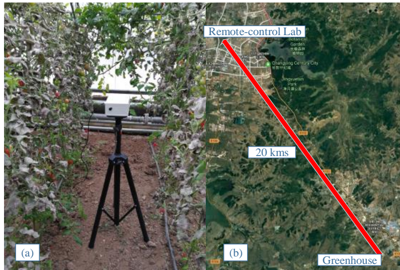
Fig. 6 – Experimental setup of the sensor node in the greenhouse (a) and geography view of the system (b)
