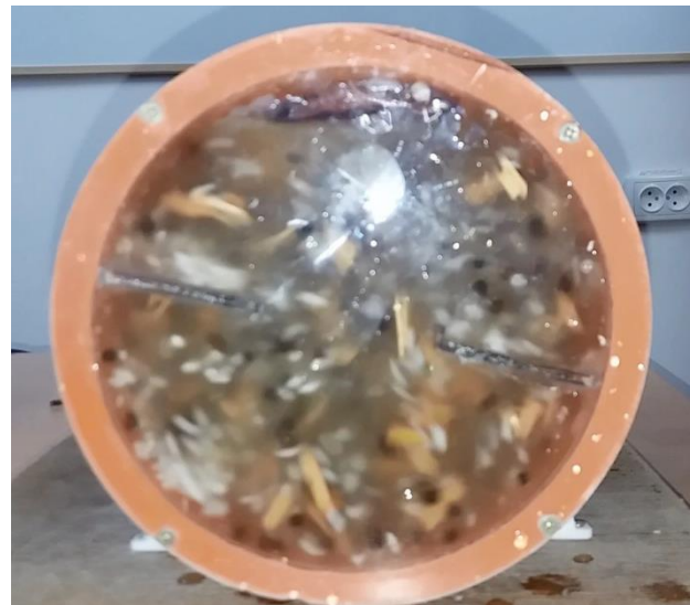
Fig. 7.- An example of the trajectory of substrate particles movement (angular velocity of the digester rotation 0.1 rad/s, inner radius 2 dm)
