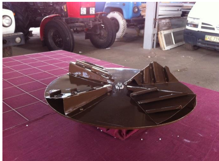
Fig. 2 - Upgraded centrifugal spreader disc
