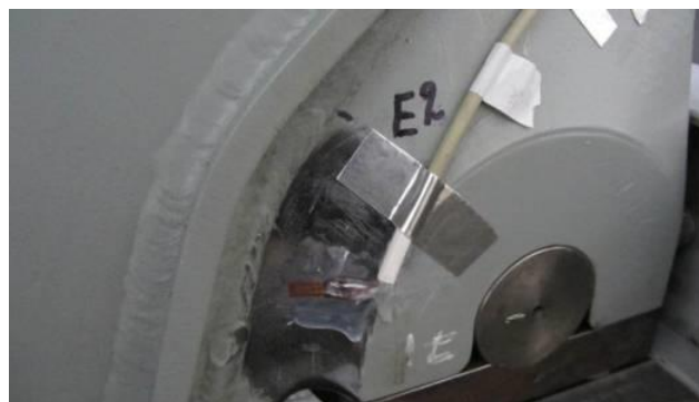
Fig.3 – Detail of strain gauge application
