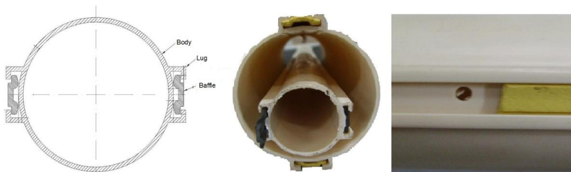
Fig.1 - Section of infiltrating irrigation tube
