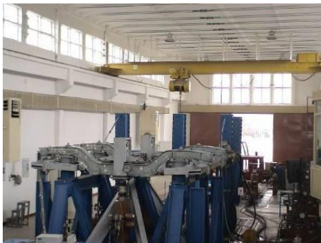
Fig. 5 – Mounting made on the Hydropulse type installation for carrying out the dynamic fatigue tests
