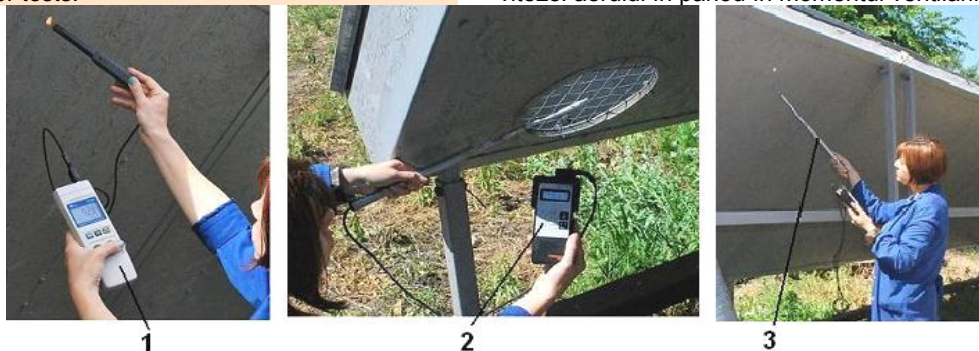
Fig. 2 - Measuring the temperature and the air speed
