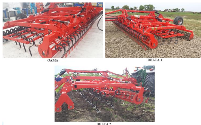
Fig. 3 - The prototype vibro-combinator SANDOKAN 2 equipped with the three types of active parts (GAMMA, DELTA1, DELTA2)
