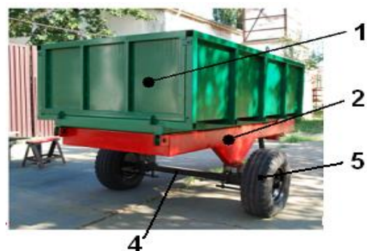
Fig. 1 – Stand for tyre testing, STP , equipped with tyres for testing 1. shutter; 2. assembled chassis; 3. body shell; 4. drivetrain; 5. tyre to be tested
