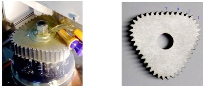
(a) Shaping process (b) Third-order elliptical gear obtained by machining experiments
