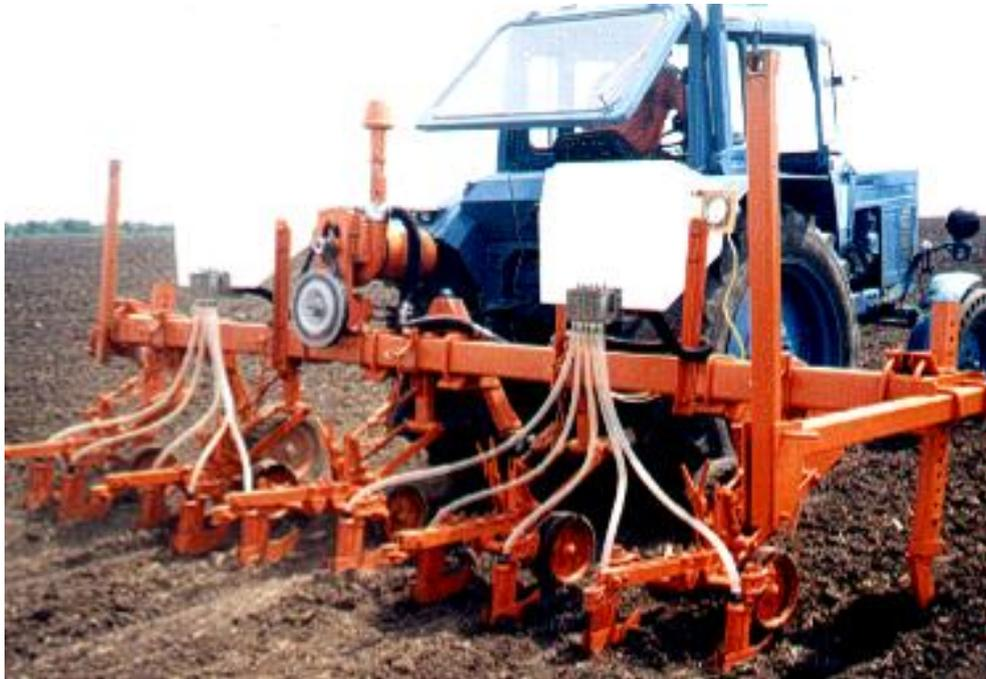
**Fig. 5 - Universal machine "seeder - cultivator"**
