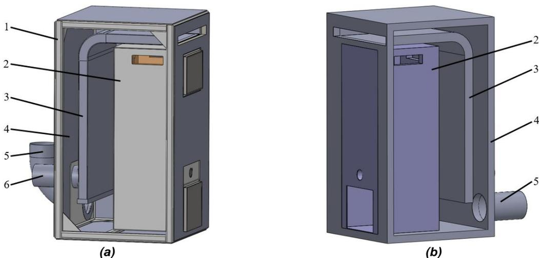
**Fig.3 - Greenhouse heating equipment (lateral wall hidden): (a) original design; (b) simplified design, for CFD simulation;**
