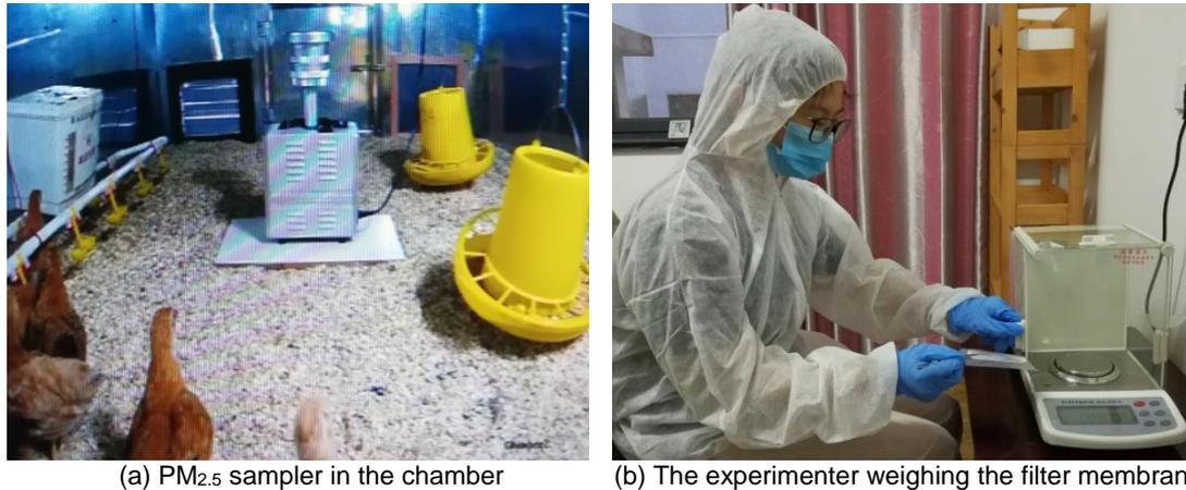
(a) PM<sub>2.5</sub> sampler in the chamber
