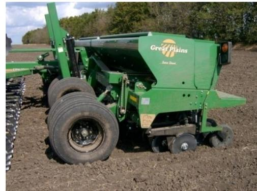
**Fig. 2 - The components of the mechanical seed drill CPH 2000 for direct seeding with the tractor Case Puma 195: battery of disc knives (a), mechanical seed drill (b)**
