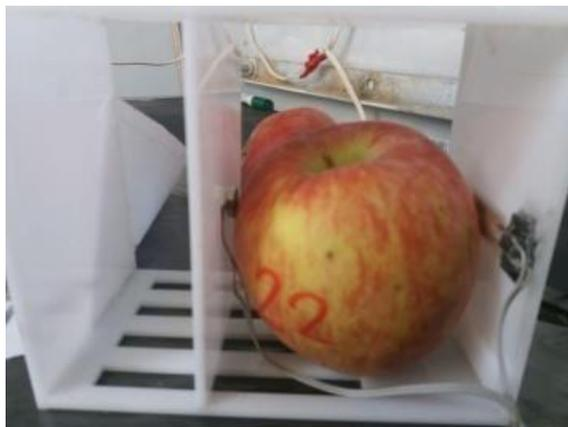
Fig.1- Non-destructive set-up to evaluate bruises
