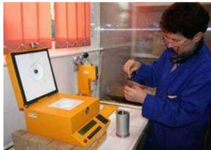
**Fig. 4 – Calorific power test / Determinarea puterii calorice**
