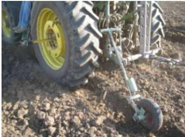
**Fig. 2 - Measuring of actual and theoretical velocity of tractor / Merenje stvarne i teoretske brzine traktora**
