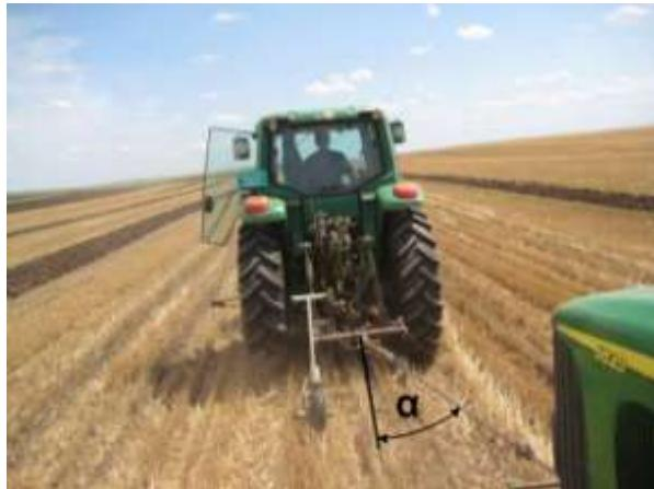
**Fig. 1 - Measuring of oblique traction of tractor on stubble / Merenje kose vuče traktora na strnjici**
