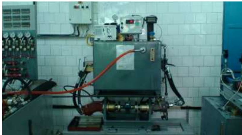
Fig.1. a - Secondary sector of the mechatronic hydraulic converter - laboratory model/ Secundarul convertizorului hidraulic mecatronic -model de laborator
