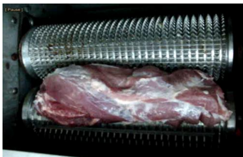
Fig. 1 - Four roller tenderizer machine (with pyramidal cutting prongs)
