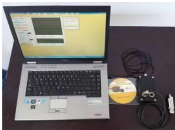
Fig. 2 - Measuring instruments for UV-C radiation intensity
