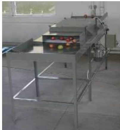
Fig. 1 - Installation for the decontamination of external surfaces of horticultural products, IDPH
